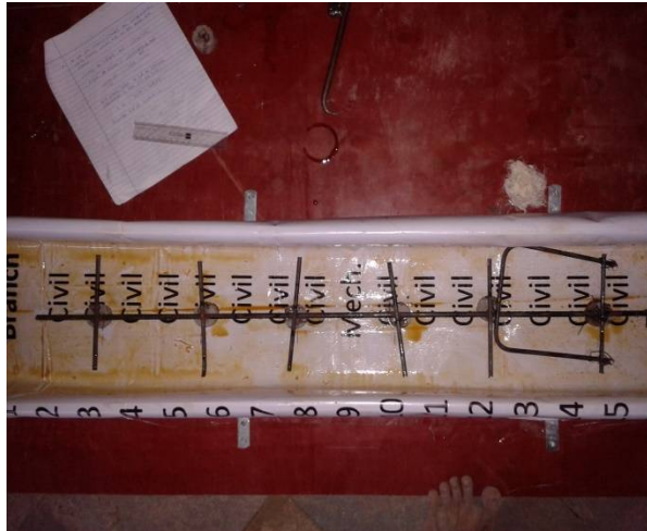
Fig (D) Mould preparation for slab 2 with reinforcement details.
